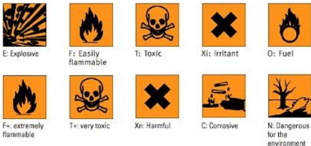
Fig. 6.13.2: Chemical hazard safety signs
