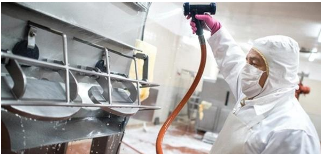
Figure 2.1.23 Pressure cleaning in Equipment (CIP)
