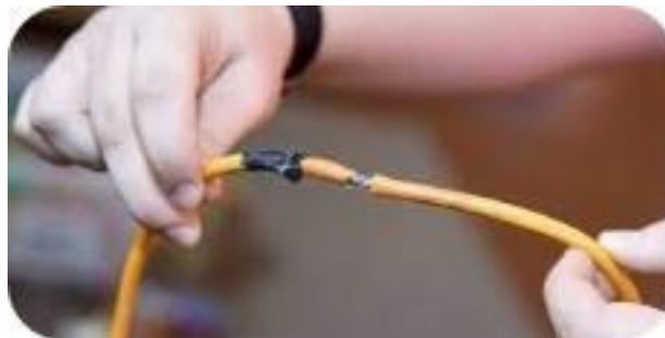
Figure 2.1.52 Damaged electrical wire
